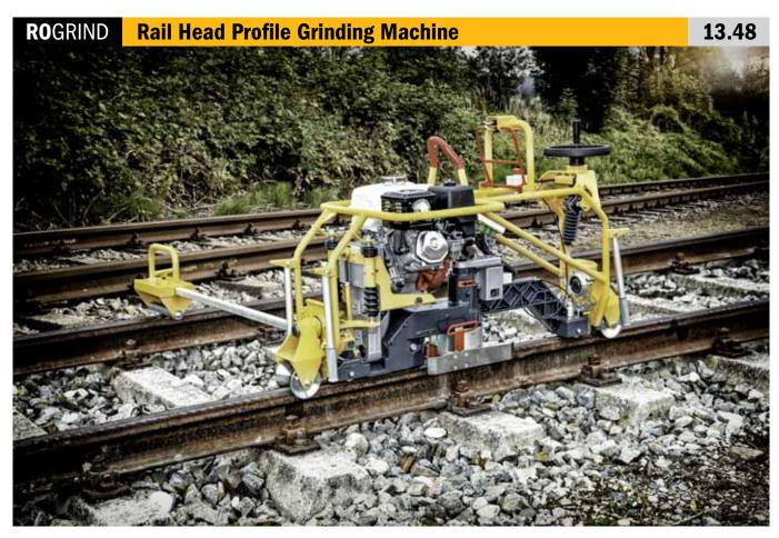
For true-to-form grinding of the rail head after welding work to restore a perfect profile
