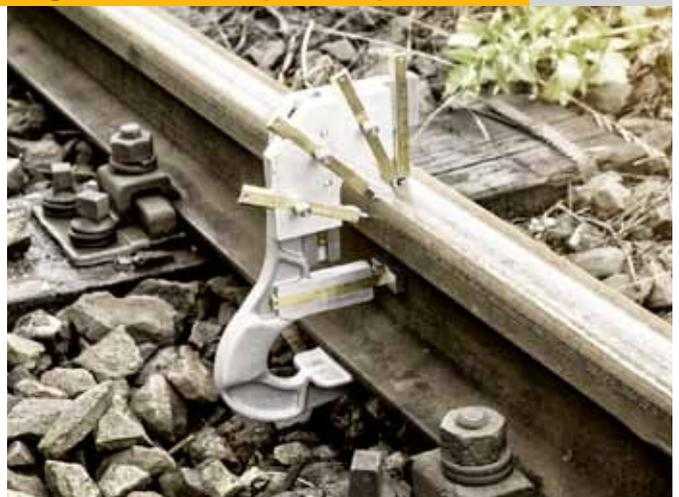
**For checking measurements L + L1 during build-up welding work in switches and crossings**
